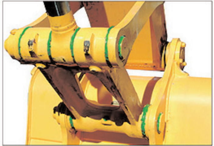
The green grease is easily visible on this excavator bucket bush and pin assembly preventing dust and moisture damage.
