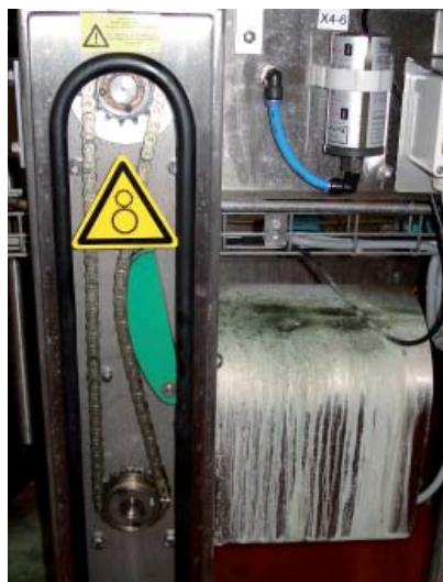
Image left and right: simalube lubricators mounted to the outside of a machine with a clamp.
