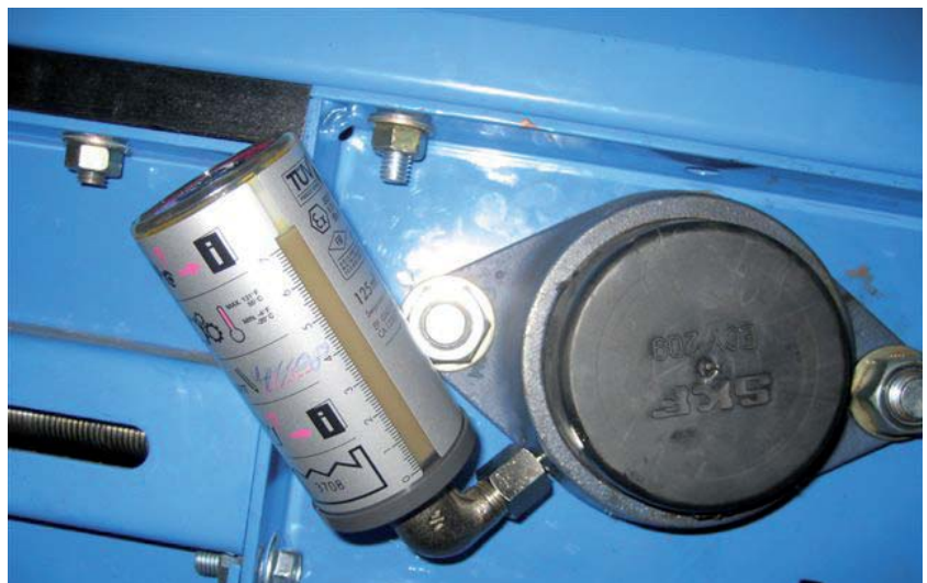
simalube mounted to a flange bearing with a 90° arch.
