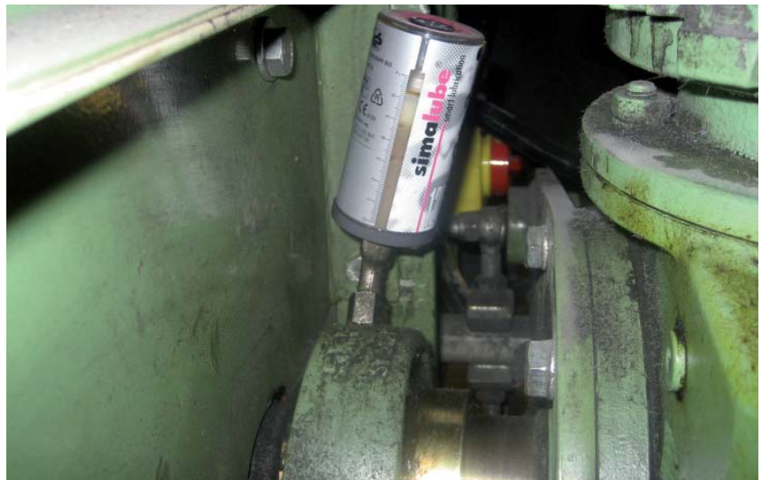
Axle driving shaft of a luggage conveyor: To mount this lubricator a 45° bent connection is used.
